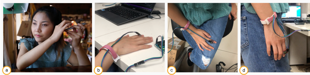
Fig. 1. (a) A visually impaired user operates a smartphone. (b), (c) and (d): Using an IMU ring to perform gestures on a table, on the top of the thigh, and on the side of the thigh to operate the phone without taking it out of her pocket
